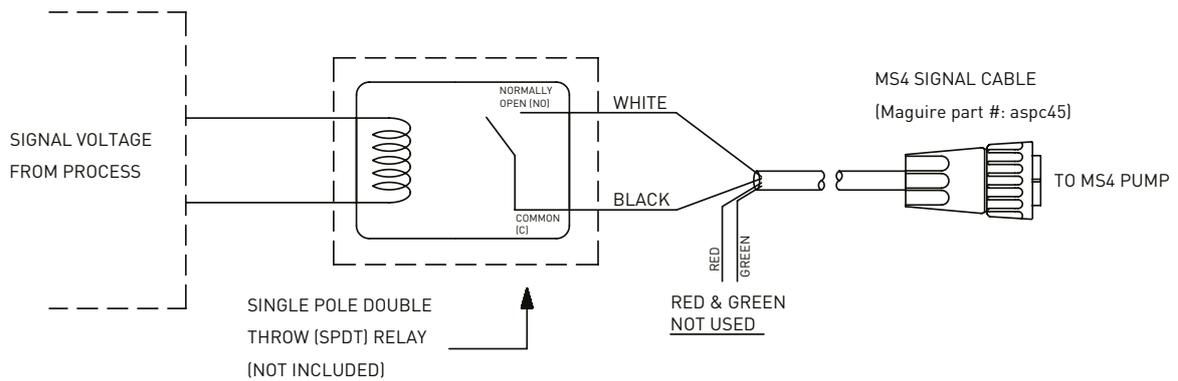
THE RELAY COIL VOLTAGE SHOULD BE CHOSEN ACCORDING TO THE PROCESS SIGNAL VOLTAGE THAT IS BEING USED
